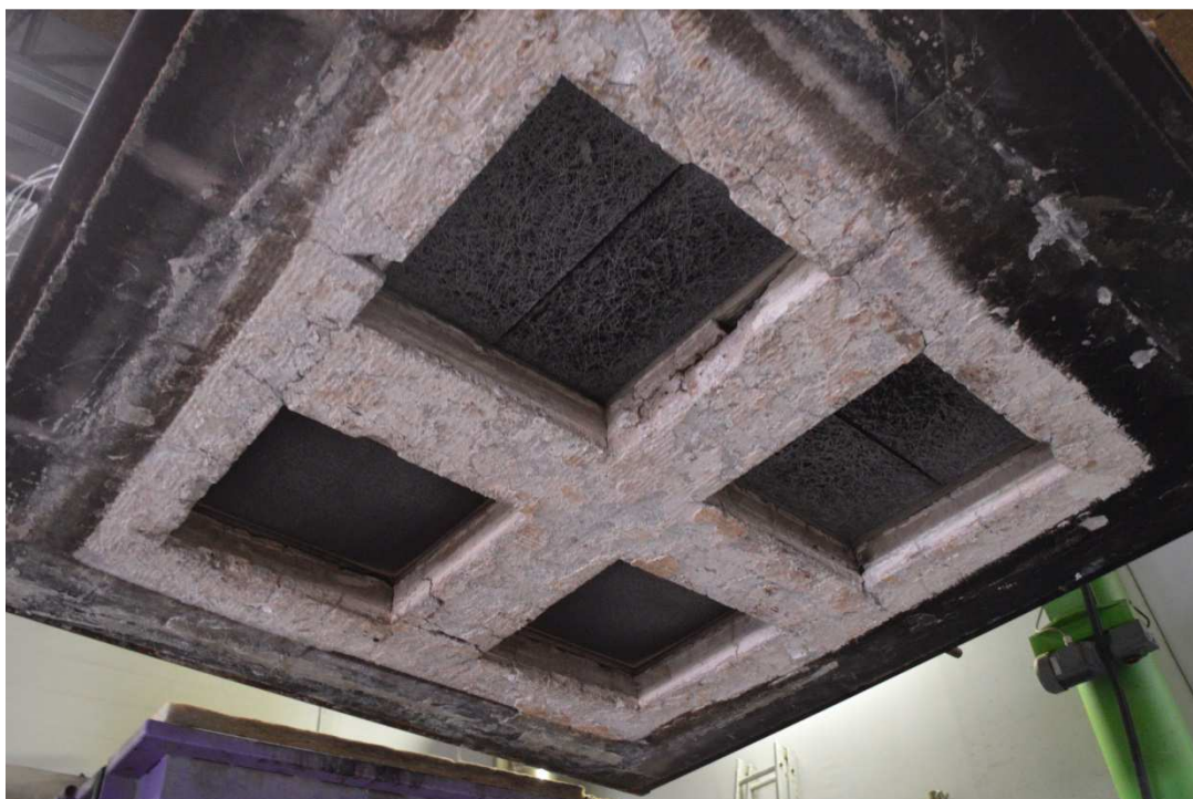
Photo No. 5 Test specimens no A1, A2, A3 and A4 from exposed side after the test
