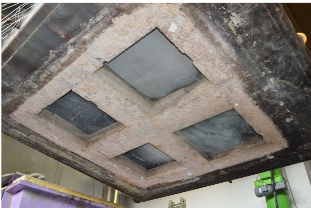
Photo No. 9 Test specimens no B1, B2, B3 and B4 from exposed side after test
