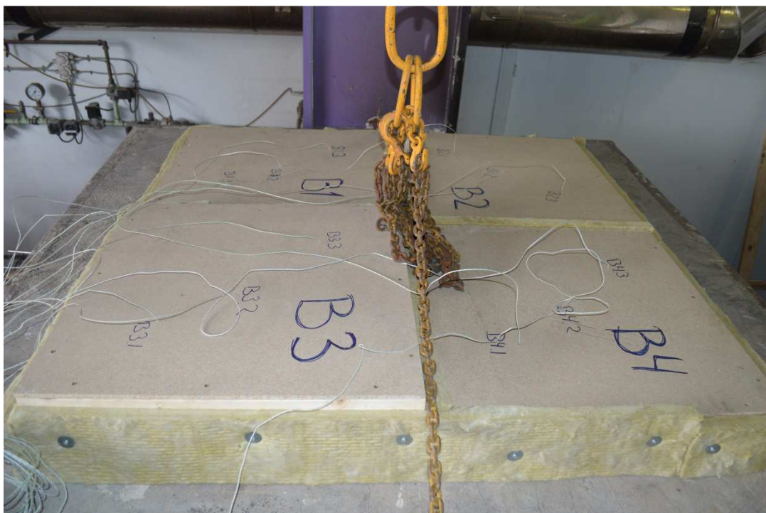
Photo No. 6 Test specimens no B1, B2, B3 and B4 from unexposed side before test
